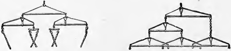
Fig. 275.—Whippetrees, for Three Horses Abreast—in Tubular Iron.
